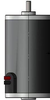
Bag Motor: 3.27" Long 1.59" Dia 0.71 Lbm
